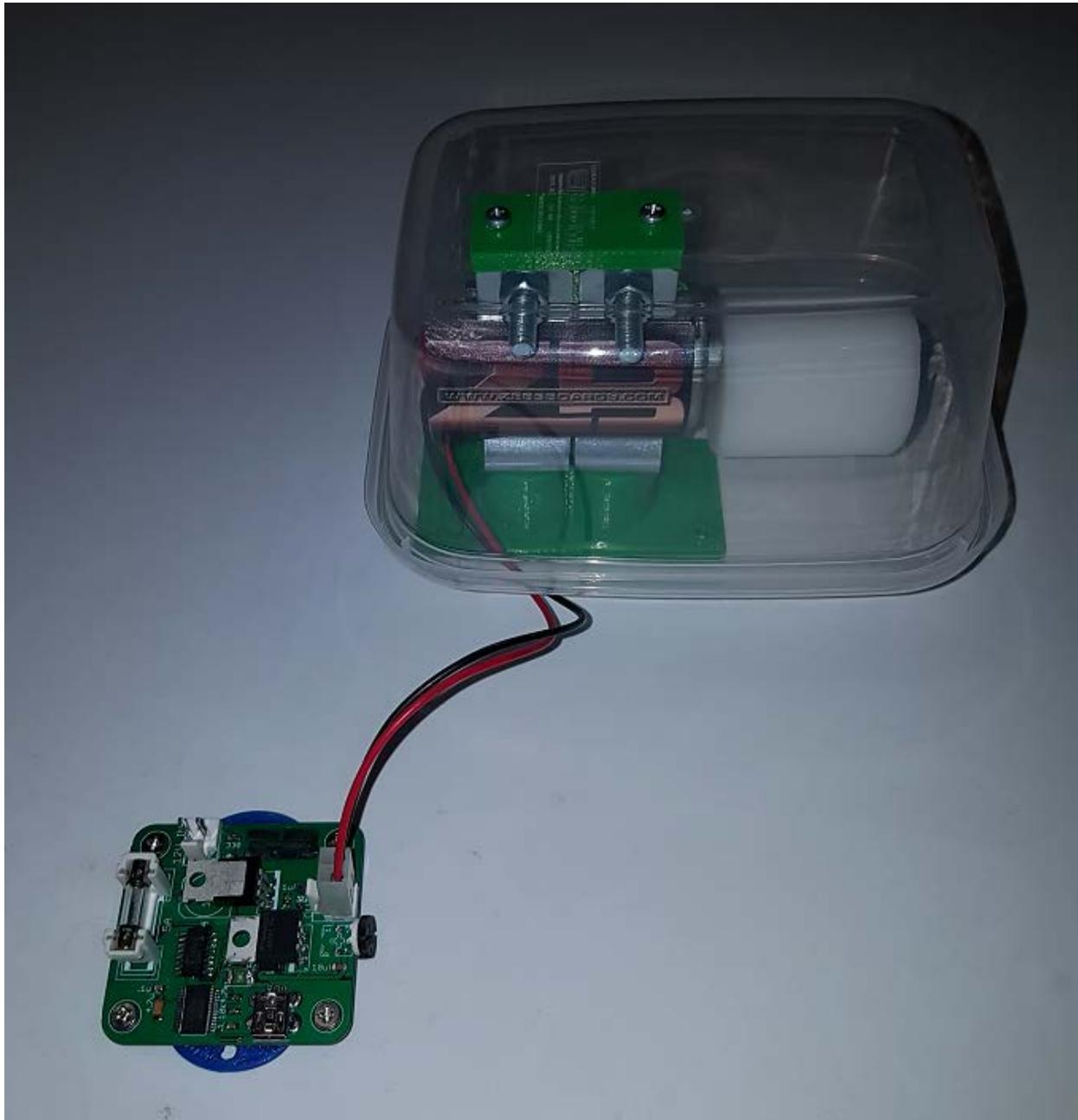
4. Crimp supplied terminal connectors to power supply wiring and install in housing as shown. Connect 9V – 12V 3A power supply (not included) to the control board.
