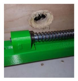
7. Pull back spring, align slide housing slots with slide block tabs and push firmly into place.
