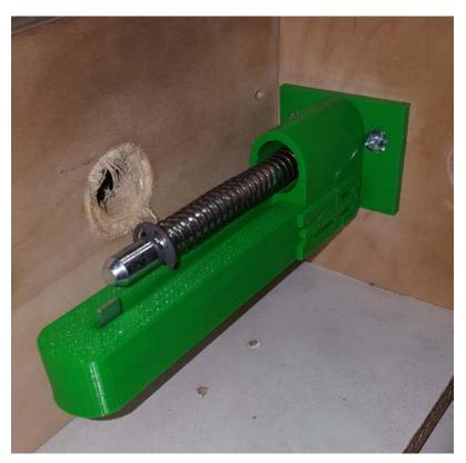
Make sure not to overtighten and damage the plunger housing plate. Screws should be tight enough to hold the ball shooter in place but not so tight as to split mounting plate.
