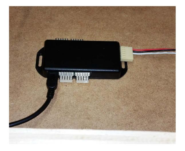
USB cable port should be toward the front of the cabinet with the plunger connector to the right side of the control box. Connect cables as shown.
