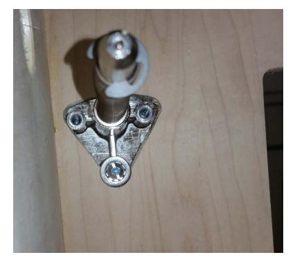
5. Mount plunger housing using supplied machine screws and star washers.
