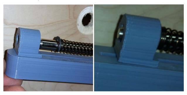
6. Push plunger firmly onto ball shooter assembly until slide is seated against pin
