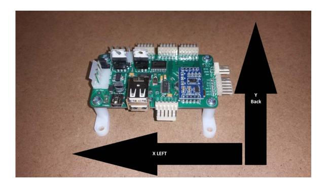
USB cable port should be toward the front of the cabinet with the plunger connector to the right side of the control box.
