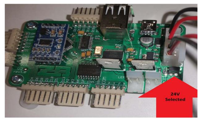
The solenoid/contactor outputs are controlled by Ports 4(Right Flipper) and 7(Left Flipper) of the onboard FTDI 245RL IC and driven by mosfet transistors capable of up to a maximum of 5A per side.
